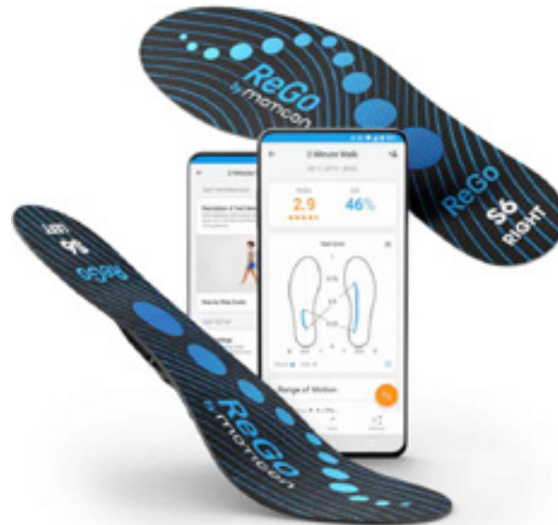
Fig. 7. The data acquisition is triggered by integrated motion detection (Image: Press image Moticon ReGo AG)
