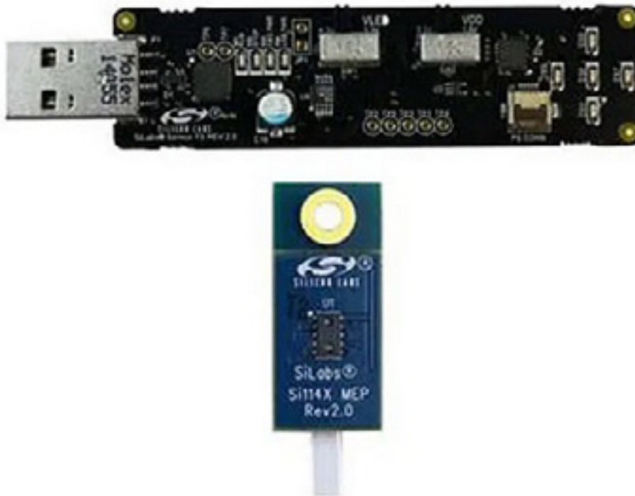
Fig. 14. The evaluation kit Si1145/46/47-M01 (USB tool stick) also from Silicon Labs is supplied with programming software. This allows access to functions of the optical sensors (Si1145-M01, Si1146-M01 and Si1147-M01). The kit can also be used to implement heart rate and pulse oximetry applications. (Image: RS Components)
