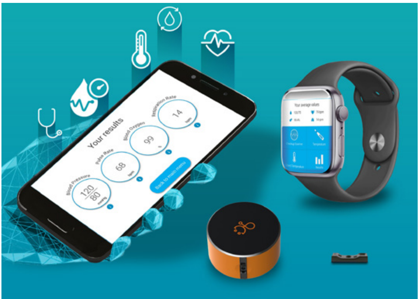
Fig. 4. A stand-alone miniature V-sensor device from Lemnan Micro Devices sends the measurement results via Bluetooth to a smartphone. There, the e-Checkup app shows the results of the blood pressure measurement. (Image: Press image Lemnan Micro Devices)
