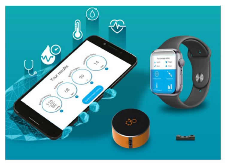
Fig. 4. A stand-alone miniature V-sensor device from Leman Micro Devices sends the measurement results via Bluetooth to a smartphone. There, the e-Checkup app shows the results of the blood pressure measurement. (Image: Press image Leman Micro Devices)
