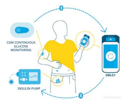
Fig. 1. The DBLG1 system adjusts the insulin delivery by means of an algorithm. (Image: Press image Diabeloop)
