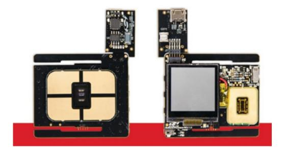
Fig. 13. Silicon Labs' Si117x biometric sensors are located in a 28-pin LGA module with 3.7mm x 7mm. There are also ECG and PPF development kits for the wrist. (Image: Press image Silicon Labs)
