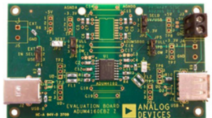
Figure 2. Development board for the IEC 60601-1 compliant ADuM4160 digital isolator iCoupler. It enables isolation of peripherals in USB applications.
