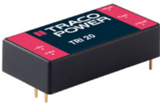
Figure 1. RS Components has the controlled DC/DC converter series TRI from Traco Power in its product range. The TRI series includes five power options: 3.5W, 6W, 10W, 15W and 20W. They offer 7,071VDC I/O isolation and peak isolation of 9000VDC up to one second duration. (Image: RS Components)
