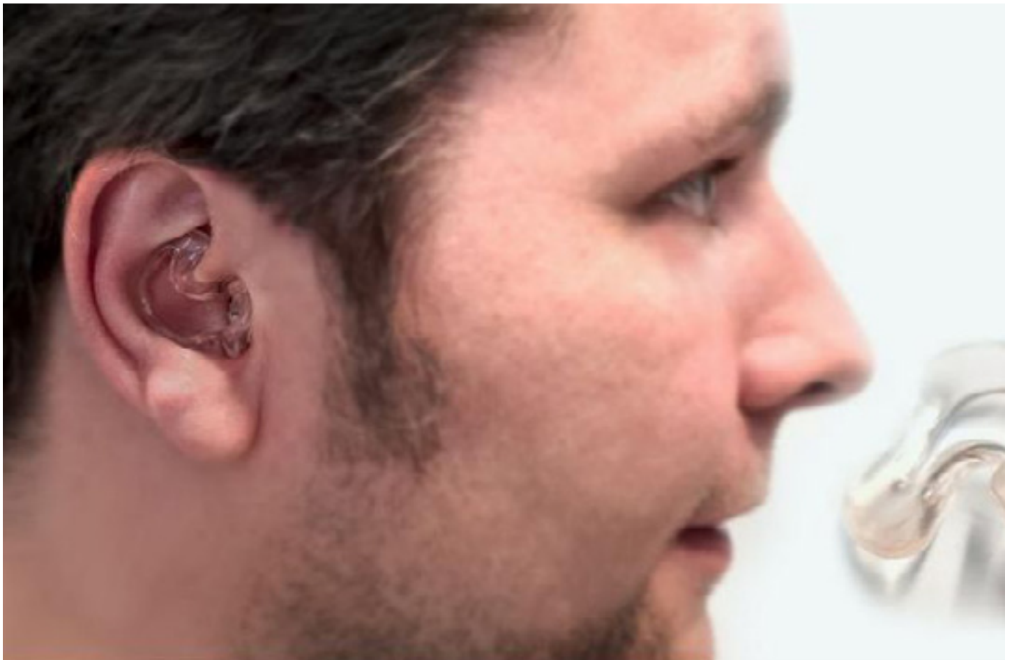
Fig. 18. The in-ear sensor for non-invasive beating-to-beat blood pressure monitoring (Image: Nadin Jurisch, press image CiS Research Institute)
