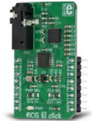
Fig. 4. The click board is suitable for use on a system with a microbus connection and is used for prototyping. (Image: RS Components)
