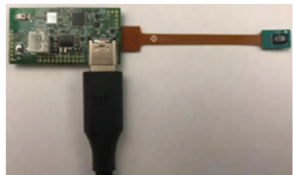
Fig. 24. The development kit is designed for in-ear applications (Image: RS Components)
