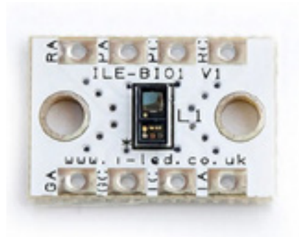
Fig. 22. The BIOFY Eco1 SFH 7050 board has mounting holes for M3 screws and has dimensions of 20.25mm x 13.7mm x 0.9mm. (Image: RS Components)
