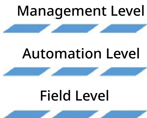
Fig. 3. Field, automation and management levels are the characteristic layers of a building automation system.
