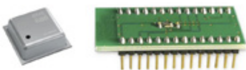
Fig. 13. On the left you can see the BME688 sensor, on the right its evaluation board. (Image: RS Components)
