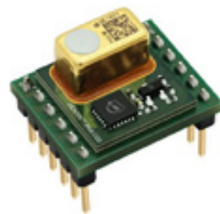
Fig. 5. Infineon's XENSIV PAS CO 2 Mini Evaluation Board enables the experimental setup and design of a CO 2 application using a 2.54mm pin header. (Image: RS Components)
