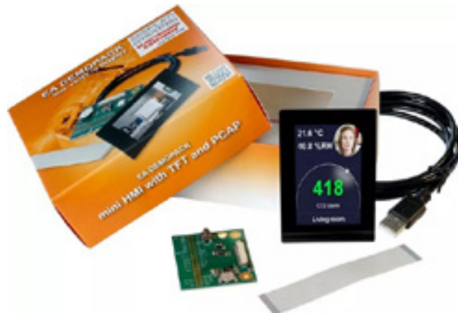
Fig. 9. The kit is suitable as a development platform for applications in the smart home sector and in the industrial environment. (Image: RS Components)
