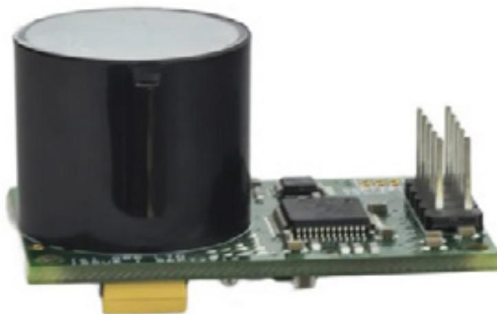
*Fig. 2. The GSS sensor measures concentrations of up to 100%. (Image: RS Components)*
