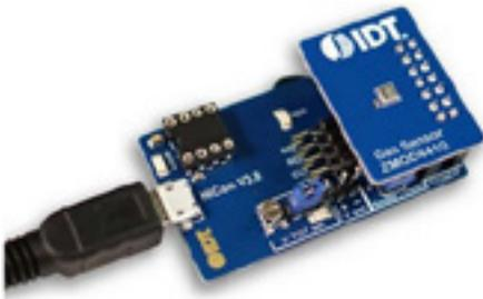
Fig. 12. The kit works with Renesas software – either with an executable ZMOD4410 GUI or alternatively with firmware programming. It allows you to connect sensor boards for different gas sensor models and integrate with other sensors via the I2C interface. (Image: RS Components)
