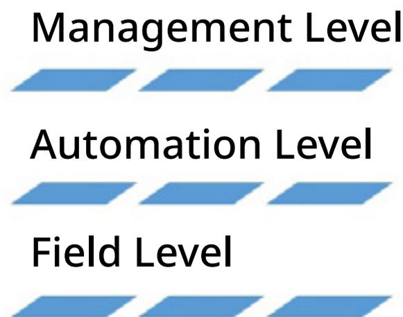
*Fig. 1. Sensors operate at field level*
