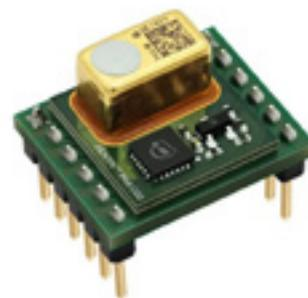
Fig. 5. Infineon's [XENSIV PAS CO<sub>2</sub> Mini Evaluation Board](#) enables the experimental setup and design of a CO<sub>2</sub> application using a 2.54mm pin header. (Image: RS Components)
