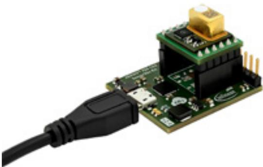
Fig. 4. Here is the compatible evaluation kit. It is called [XENSIV™ PAS CO<sub>2</sub> Sensor2Go](#) and can be used in combination with Infineon's PAS CO<sub>2</sub> Mini Evaluation Board (image below). (Image: RS Components)
