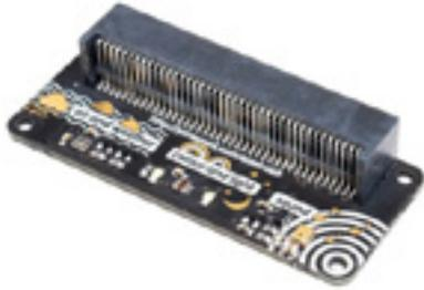
Fig. 11. The PIM355 is simply plugged onto a Micro:bit – no soldering required. (Image: RS Components)
