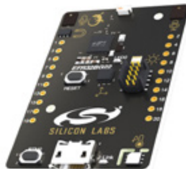
Fig. 6. The EFR32BG22 module is used in the Silicon Labs Bluetooth direction-finding solution. (Image: Press image: Silicon Labs)
