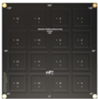
Fig. 5. The Silicon Labs Direction Finding Antenna Array used in SiLabs' Bluetooth direction-finding solution. (Image: Press image: Silicon Labs)
