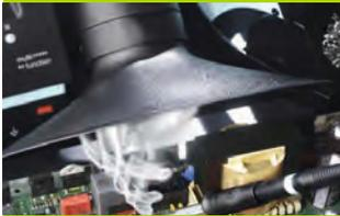
Lead free soldering produces up to 250 % more particles in the breathing zone than leaded solder. As much as 700 million small particles per cubic meter are produced, which can be transported into the alveoli.
