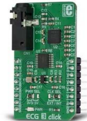
Fig. 4. The click board is suitable for use on a system with a microbus connection and is used for prototyping. (Image: RS Components)
