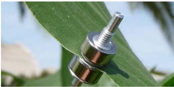
Fig. 1. The non-invasive ZIM-probe (now Yara ZIM Plant Technology) continuously measures the water supply of plants. The sensor system is applied to a leaf with two magnets and measures the cell turgor pressure. (Image: Yara Press Images)
