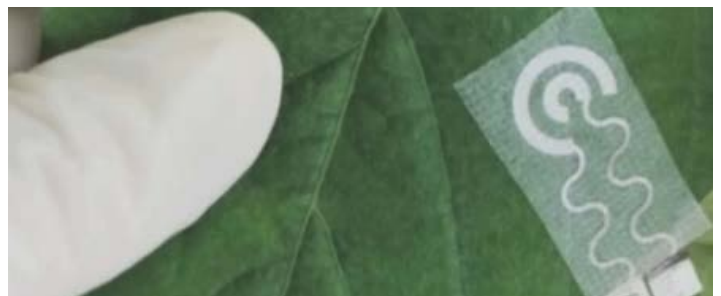
Fig. 2. The technology uses electrodes consisting of individual Ni membranes produced by established microfabrication methods. Suitable for mass production, these electrodes are the key to enabling researchers to reproducibly determine the LWC. The electrodes work by directly transferring the conductive materials to downy soy leaves using regular adhesive tape. (Images: American Chemical Society)
