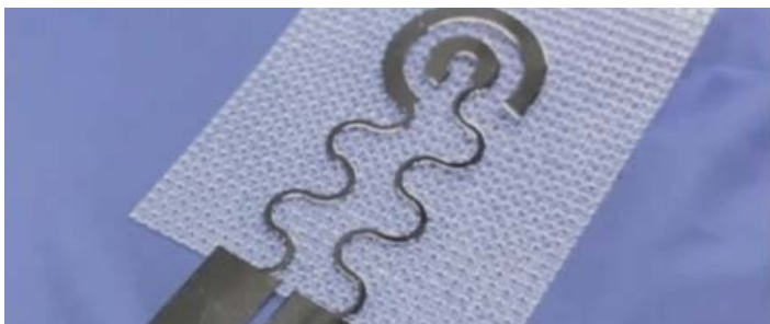
Fig. 2. The technology uses electrodes consisting of individual Ni membranes produced by established microfabrication methods. Suitable for mass production, these electrodes are the key to enabling researchers to reproducibly determine the LWC. The electrodes work by directly transferring the conductive materials to downy soy leaves using regular adhesive tape. (Images: American Chemical Society)
