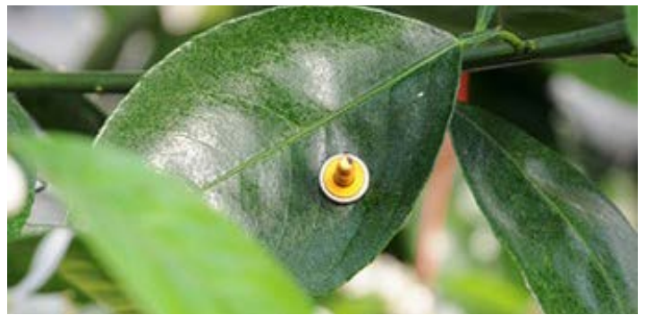
Fig. 1. The non-invasive ZIM-probe (now Yara ZIM Plant Technology) continuously measures the water supply of plants. The sensor system is applied to a leaf with two magnets and measures the cell turgor pressure. (Image: Yara Press Images)
