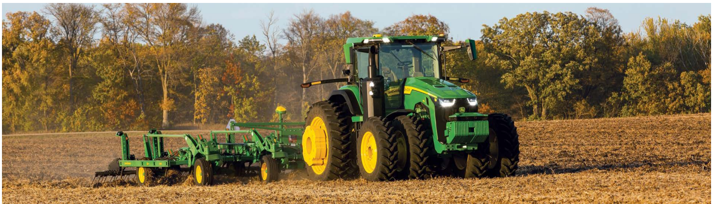
Fig. 3. A fully autonomous tractor from the manufacturer John Deere. (Image provided courtesy of John Deere)
